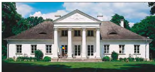
Noblemen's houses were typically single-storey buildings fronted by an imposing colomnade. Rooms flanked the central entrance hall.
