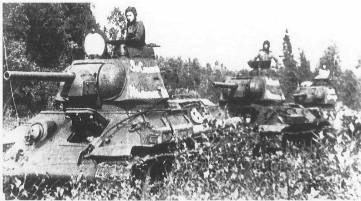
A platoon of late-model T-34/76 Model 1943 with commander’s cupola. The introduction of this cupola corrected a design flaw and finally gave tank commanders the ability to fully view the battlefield. [Courtesy of the Central Museum of the Armed Forces Moscow]
