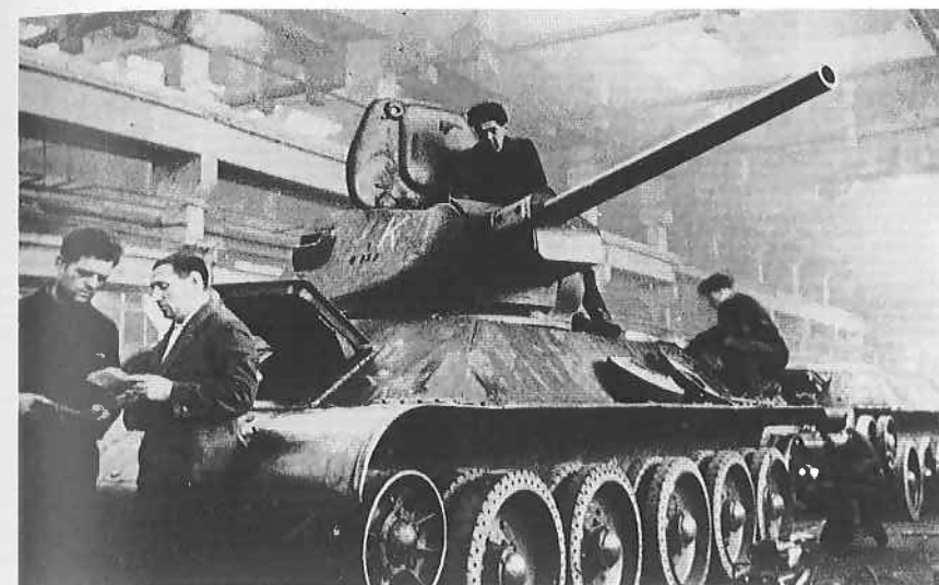
Building a T-34/76 in the Urals. A T-34/76 in 1943 cost 135,000 rubles [$25,470] and required about 3,000 man-hours to complete. A Panther cost about 129,000 Reichsmarks [$51,600] and 55,000 man-hours to complete. (Tank Museum, Bovington)
