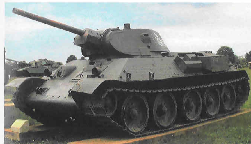
Soviet T-34/76 Model 1941 medium tank with welded turret and rubber-ribbed road wheels. This tank was a great shock to the Germans in 1941 and prompted the development of the Panther. [Author's collection]
