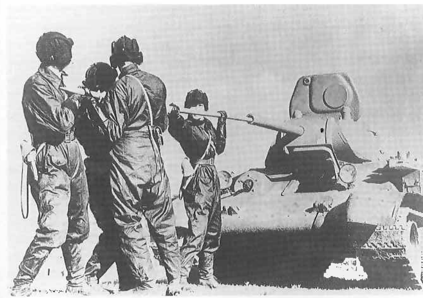
A T-34 crew “punches the gun tube” in order to clean the F-34’s gun barrel of carbon residue after firing a significant number of rounds. [Tank Museum, Bovington]
