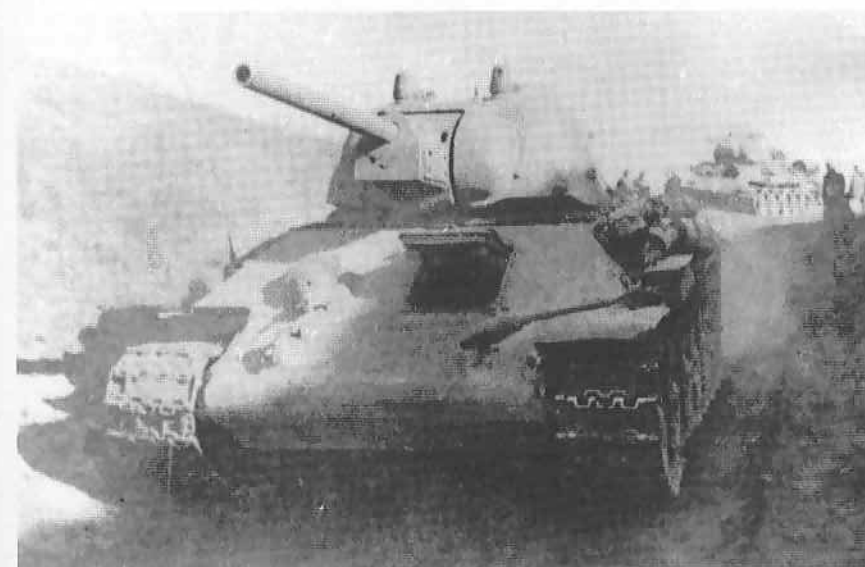
The large driver's hatch on the T-34 made ammunition loading easier and offered better chances for escape in the event of the tank being hit. (Courtesy of the Central Museum of the Armed Forces Moscow)
