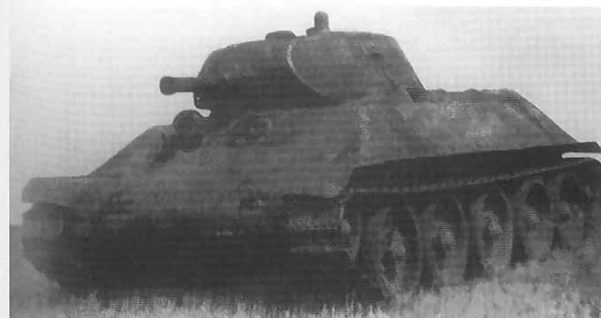
A prototype T-32 medium tank, armed with the L-11 76.2mm gun. Koshkin built this prototype in 1939 on his own initiative and it led to the improved T-34 design. (Kharkov Morozov Machine Building Design Bureau KMDB)
