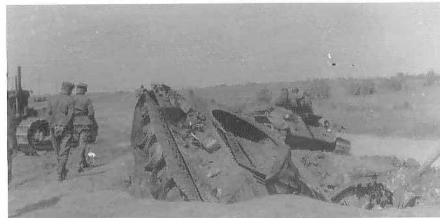
Two destroyed T-34 Model 1941 tanks. It was not uncommon for the T-34's own ammunition to "cook off" after an internal fire and blow the turret off. [Nik Cornish WH617]
