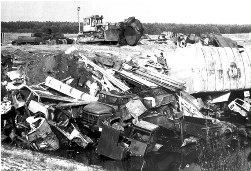
Figure 12.1. Radioactive waste disposal pit for contaminated vehicles. (Courtesy: Chernobylinform.)
