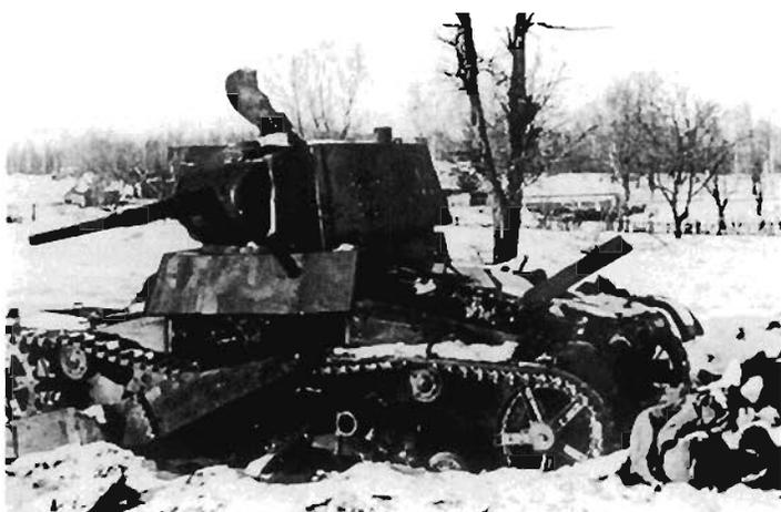
*A knocked out Soviet T-70 light tank which appears to have suffered an internal explosion after being struck by a German shell. The T-70 was designed to be primarily an infantry support tank although it did not have a sufficiently heavy main gun to be more than marginally adequate in this role. It was lightly armored and the shells of Panzer IIIs and Panzer IVs could penetrate its frontal armor even at moderately long range. (Credit National Archives)*
